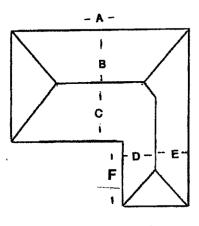
$A \times (B + C) + F \times (D + E) = TOTAL ROOFING AREA$
