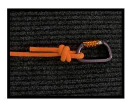
A Scaffold knot is essentially a double overhar knot that has been applied to a bight of rop?
