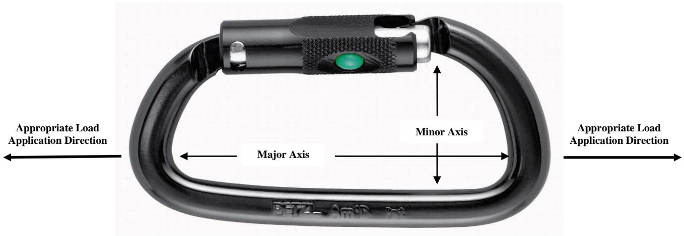
**Warning:** Carabiners represent a quick and easy way of establishing a rope access connection however, to avoid compromising a carabiner's greatest listed strength, they should always be loaded in a single direction along the major axis with the gate securely closed.
