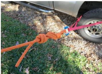
*Establishing an anchor point around an axle or tire rim is an effective means of securing a lifeline however, should incorporate the use of tubular webbing to prevent shear damage to a rope.*
