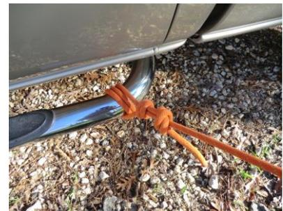
**Examples of Appropriate Fixed Anchors:** Trees, fence posts, deck posts, heavy shrubs, fire hydrants, anchor barrels and vehicles.
