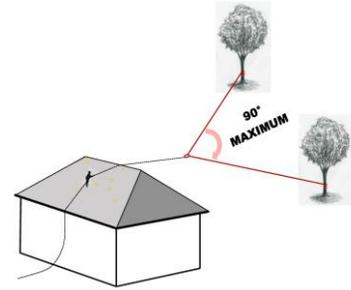
**Weight Based Anchors**- utilized only in situations where no suitable fixed anchors are present. Should be appropriately placed directly under the opposing eave of the roof slope to be inspected and consist of a weight approximately equal or greater to that of the roof climber.
