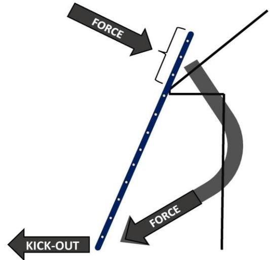
**Ladder Kick-Out** – is the leading cause of ladder access related injuries that occurs when the dynamic forces applied to the ladder exceed the traction of the ladder’s base footing. The application of climber’s weight to any rung located above the rail contact points at the eave of the roof can cause catastrophic ladder failure.
