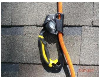
**WARNING:** Ascenders can fail with as little as 600 lbs of load force therefore are not approved by manufacturers to use alone as a primary belay device!
